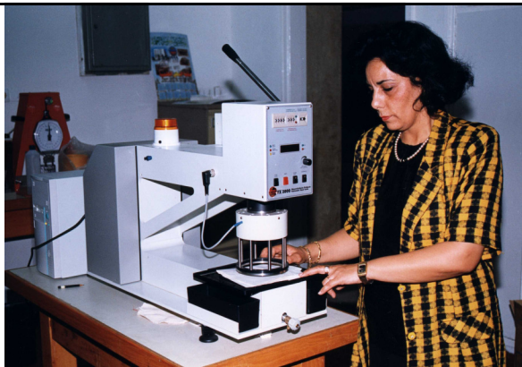
Hydrostatic pressure tester (water permeability)
